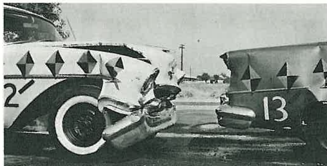
Results of a steel against steel impact at 17 mph.
