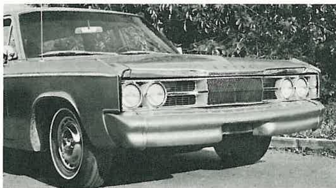
Results of a vinyl against vinyl impact at 18 mph.
